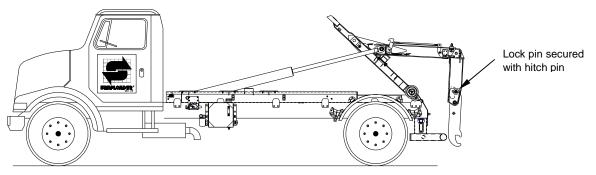
2. Tilt the telescopic arm toward the cab (left control lever forward). See Fig. A (Pg. 3-1).
