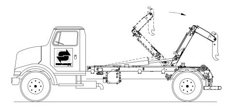
4. Continue to tilt telescopic arm rearward until the dump cylinders are fully extended. Replace lock pin and secure with hitch pin.
