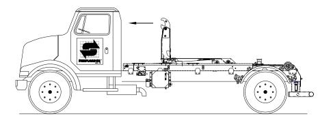
4. With the telescopic jib fully extended in the transport position (as shown); replace the lock pin and secure with hitch pin.
