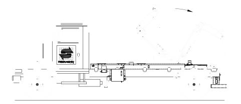
4. Continue to tilt telescopic arm rearward until the dump cylinders are fully extended. Replace lock pin and secure with hitch pin.
